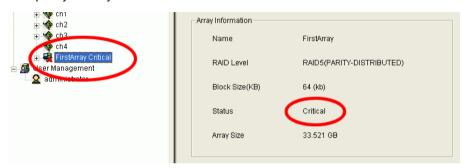
Figure 72. An Array in Critical condition highlighted in Tree View (left) and shown in red in Information View (right).
